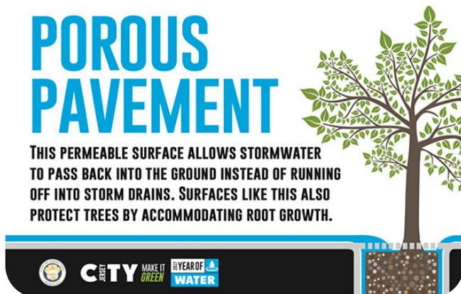
The [porous pavement](#) allows rain to enter the ground instead of flowing into sewers. This is part of the smart green infrastructure plan to manage stormwater runoff while also providing a safe and accessible route for all users.
